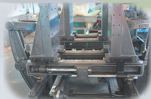
4 中央支承模架 Central supporting frame for the mould
