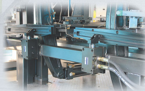
5 移模速度控制阀 Speed control valves for mould's movement
